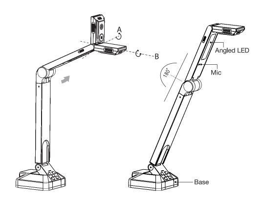
The camera head can flip up and down on the A axis and can rotate 90° counter-clockwise or 270° clockwise on the B axis .
